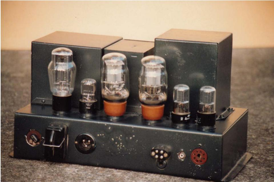
1950. A *Williamson* amplifier marketed by Goodsell, England. This variant incorporates an auxiliary rectifier 6X5 valve (2<sup>nd</sup> from left) for powering attached pre-amps etc.
