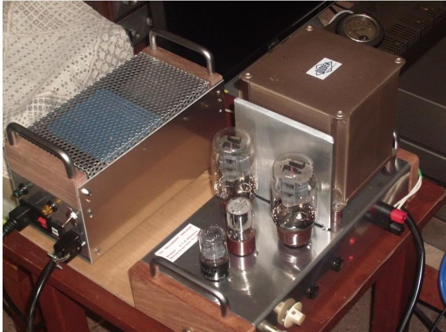
Three more power amplifier modules with output transformers by Beacon (N.Z.), Partridge (U.K.) and Bramco (Aust.)
