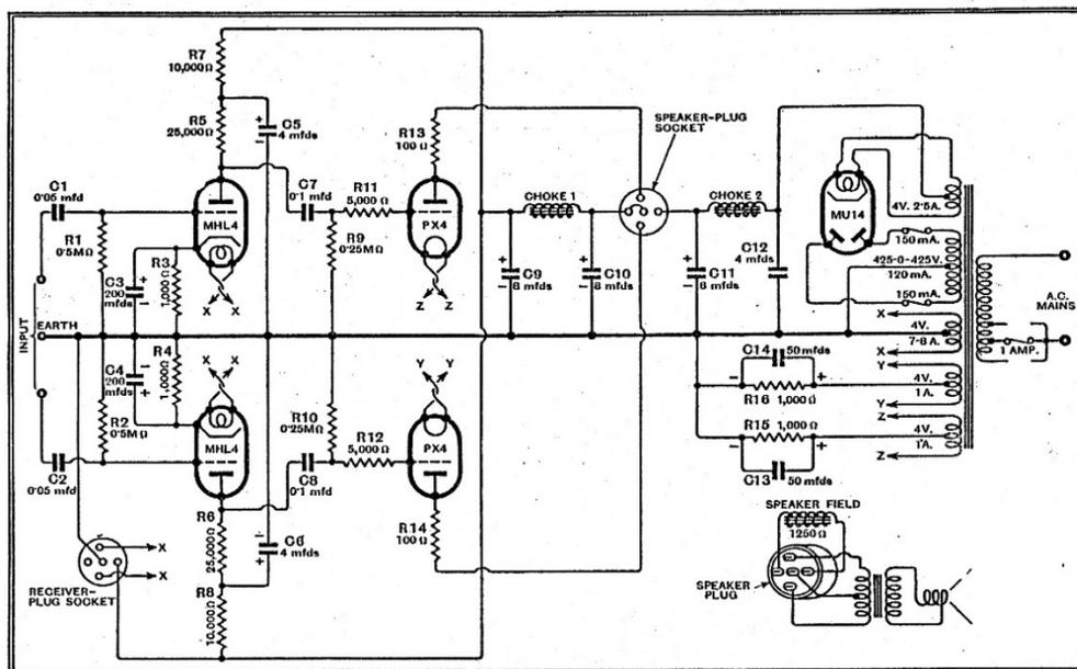
1934. The circuit for the *Wireless World Quality Push Pull Amplifier*. An additional pre-stage to provide the push pull drive was also described. Output transformer to be chosen by the user, according to the loudspeaker to be used.
